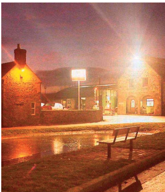
Badly mounted floodlight illuminates neighbouring premises, Peak District
